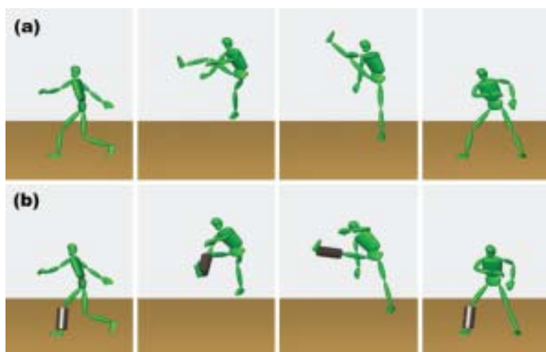
Fig. 10. Jump Kick: (a) original motion (b) when a load is attached (dynamic-filtered).
